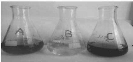
Fig 1- Digital photographs of (A) Flower extract, (B) 1mM ZnSO 4 , (C) ZnO nanoparticles with H. rosa-sinensis
